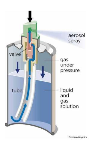
Push down on the actuator which moves the stem down.
